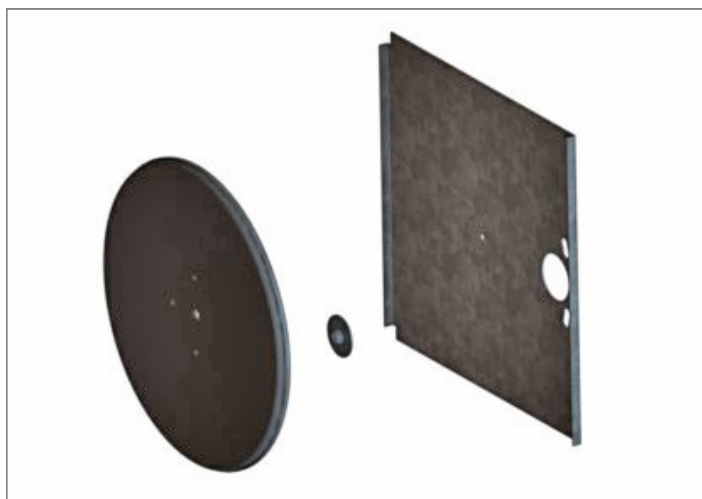
Step 2: Remove air caster and inlet plumbing from tray.
